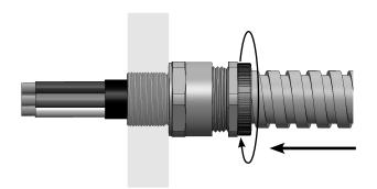
5. Tighten the seal nut (3) using a spanner until resistance is felt (when the seal engages the cable) and then tighten further one full turn with a spanner.
